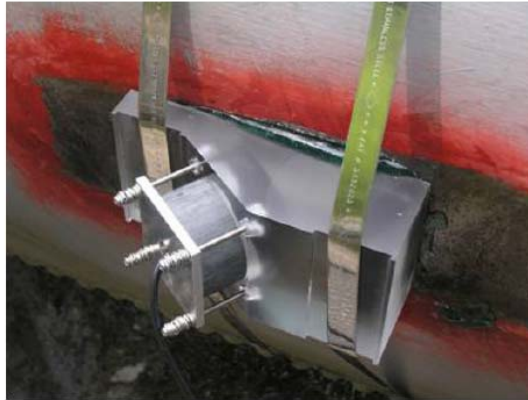
Fig. 4.4. Ultrasonic transducer and wedge which are installed on the outside surface of the pipe.
