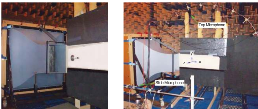
Figure 13: Experiment setup in the anechoic chamber.
