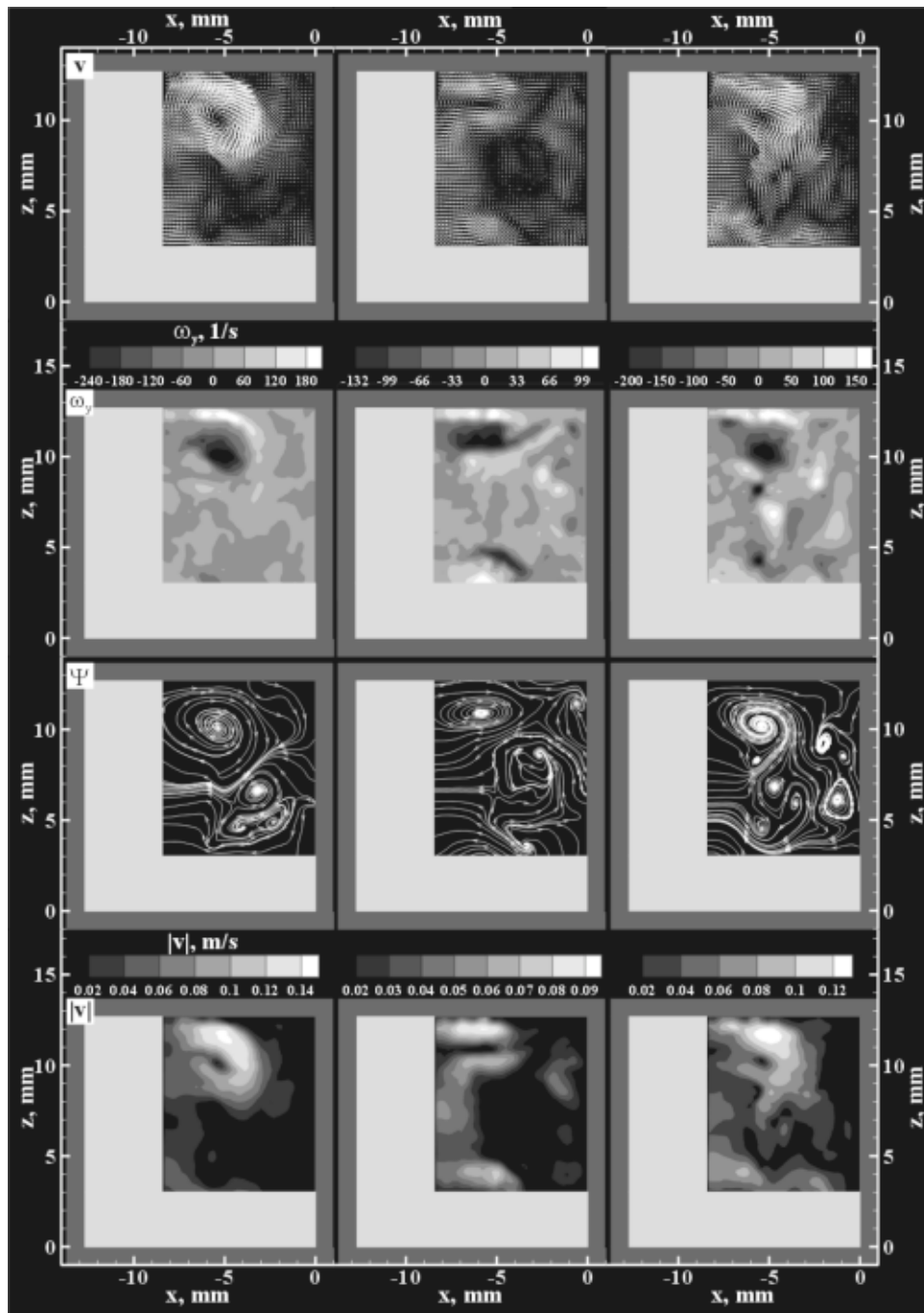
Fig. 8 Cross-flow plane: Instantaneous flow fields at Re=872 . From top to bottom: velocity vector field, out-of-plane vorticity contours, velocity streamlines, and velocity magnitude.
