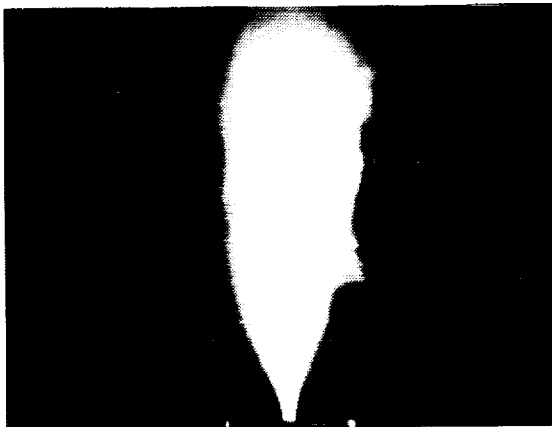
e) \dot{m}_{N_2} = 9.07 \text{ g/s} (0.020 \text{ lb}_m/\text{s}) ; \dot{m}_{N_2O} = 9.07 \text{ g/s} (0.020 \text{ lb}_m/\text{s})
