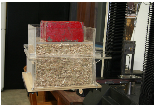
Fig. 2. Direct shear cell filled with chopped biomass with preconsolidation load. Experiments were conducted by applying uniformly distributed load on the biomass using a 9 mm thick acrylic sheet over the biomass.
