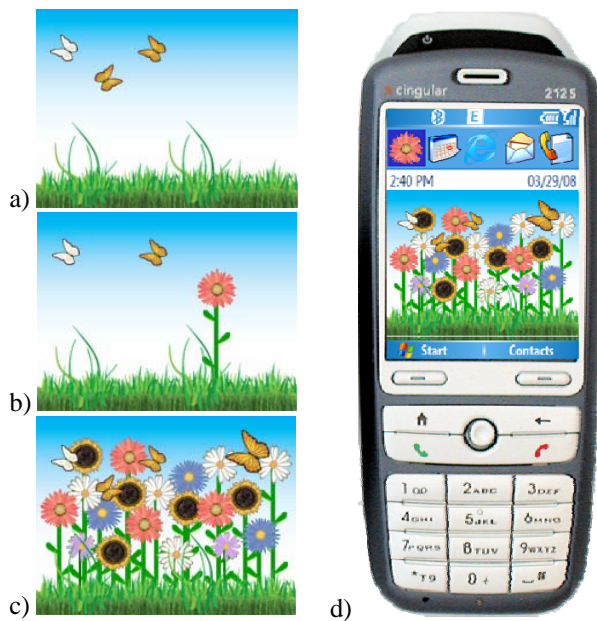
Figure 1. UbiFit Garden's Glanceable Display. a) at the beginning of the week; b) after one cardio workout; c) a full garden with variety; and d) a full garden on the background screen of a mobile phone. Butterflies indicate met goals.
