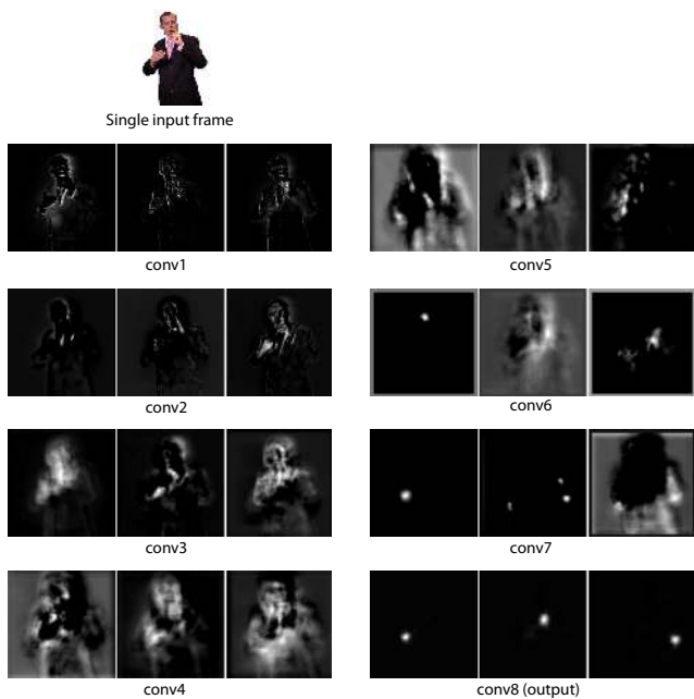
Figure 5. Sample activations for convolutional layers. Neuron activations are shown for three randomly selected channels for each convolutional layer (resized here to the same size), with the input (pre-segmented for visualisation purposes) shown above. Low down in the net, neurons are activated at edges in the image (e.g. conv1 and conv2); higher up, they start responding more clearly to body parts (conv6 onwards). The outputs in conv8 are shown for the right elbow, left shoulder and left elbow.
