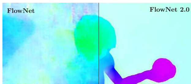
Figure 1. We present an extension of FlowNet. FlowNet 2.0 yields smooth flow fields, preserves fine motion details and runs at 8 to 140fps. The accuracy on this example is four times higher than with the original FlowNet.
