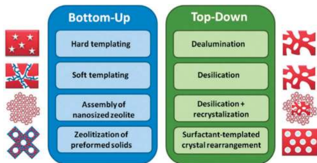
Fig. 18 Bottom-up and top-down approaches to hierarchical mesoporous zeolites. (Reproduced with permission from ref. 83, Copyright Wiley-VCH, 2014.)
