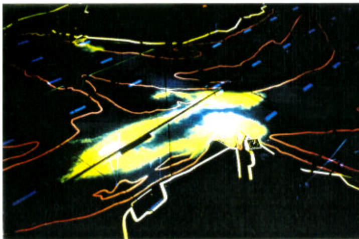
Figure 2.1 Visualization with dye to study water flow in a river model (Courtesy Delft Hydraulics)
