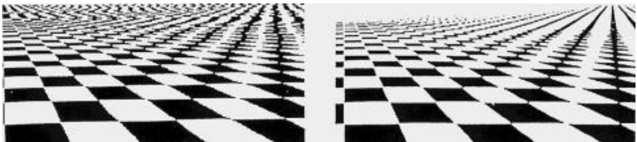
Figure 4.14 Aliasing in texture mapping - left: with point sampling; right: with digital frequency filtering (Heckbert '86)
