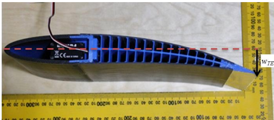
Figure 2. FishBAC wind tunnel test model showing deflected shape
