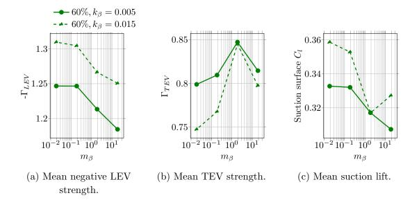
FIG. 26: Plots of various physical quantities characteristic of dynamic behavior in the flap-vortex interaction regime averaged over one time period for 60% location, and varying mass ratio and stiffness.
