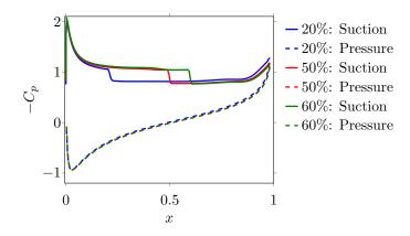
FIG. 10: Comparison of the pressure dam effect at different flap locations via mean  $C_p$  distribution for  $m_\beta = 1.875, k_\beta = 0.0015$ .
