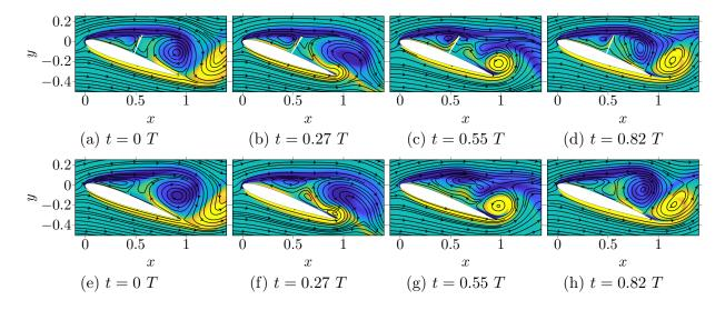
FIG. 2: Vorticity contours depicting vortex shedding from the leading and trailing edges of the airfoil for a representative case of  $k_{\beta} = 0.001$ ,  $m_{\beta} = 1.875$  and 50% location (top row) and the flap-less baseline airfoil case (bottom row) at four time instants in a lift cycle.
