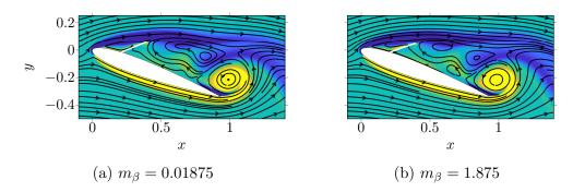
FIG. 15: Demonstration of insubstantial variations in TEV-induced reverse flow for upstream 20% flap location and  $k_{\beta} = 0.0015$  via vorticity contours and superimposed streamlines at t/T = 0.55.
