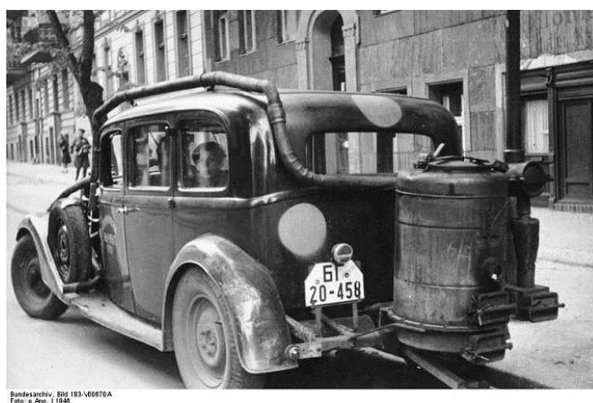
Figure 1. A WWII car with woodgas generator [4].
