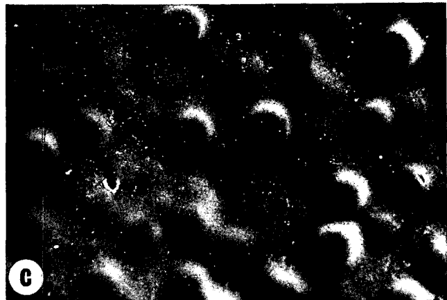
Fig. 2—Photographs of a cleaned membrane skin after reverse osmosis of Gouda cheese whey and skim milk with a fluidized bed after a process time of 150 hr: (A) The damage to the membrane skin caused by lead beads ( d = 3 mm, \epsilon = 0.95 ), enlargement 150x. (B) Deposits in the damaged parts after the use of lead beads ( d = 3 mm, \epsilon = 0.95 ), enlargement 1000x. (C) Corrugated membrane skin after the use of glass beads ( d = 3 mm, \epsilon = 0.8 ), enlargement 80x.
