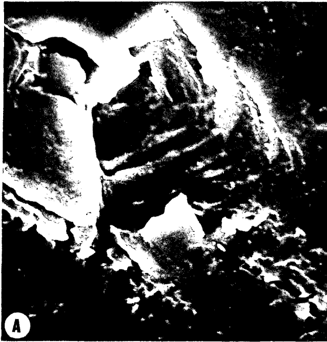
Fig. 2—Photographs of a cleaned membrane skin after reverse osmosis of Gouda cheese whey and skim milk with a fluidized bed after a process time of 150 hr: (A) The damage to the membrane skin caused by lead beads ( d = 3 mm, \epsilon = 0.95 ), enlargement 150x. (B) Deposits in the damaged parts after the use of lead beads ( d = 3 mm, \epsilon = 0.95 ), enlargement 1000x. (C) Corrugated membrane skin after the use of glass beads ( d = 3 mm, \epsilon = 0.8 ), enlargement 80x.
