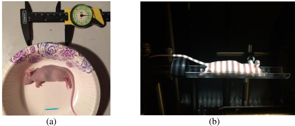
Figure 5.1: (a) Photo of the nude mouse and the fluorescent target (the blue bar at the bottom of the picture). (b) The mouse illuminated by the pico-projector for the surface scan.
