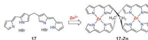
Fig. 5 Proposed \text{Zn}^{2+} sensing mechanism using the 3,3'-bis(dipyrren) salt 17 .
