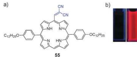
Fig. 23 (a) Chemical structure of CN^- probe 55 ; (b) images of probe 55 before (left) and after (right) addition of CN^- under a portable UV lamp. Reprinted with permission from ref. 46, copyright (2013) Royal Society of Chemistry.
