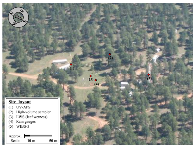
Figure 1. Aerial overview of BEACHON-RoMBAS field site at the Manitou Experimental Forest Observatory located northwest of Colorado Springs, CO. Locations of all instruments and sensors discussed here are marked and were located within a 50 m radius. Figure adapted from Fig. 1a of Huffman et al. (2013).
