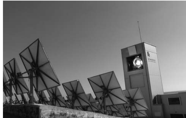
Fig. 2 The Cyprus Institute’s “iStore” receiver in operation at the research and testing facilities of the Institute at Pentakomo, Cyprus
