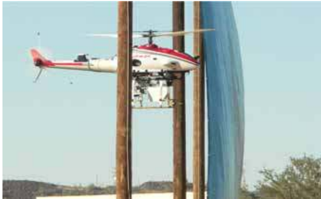
Figure 1: The helicopter platform we used to test collision avoidance is flying autonomously in between two poles 10 m apart. The rotor span of this helicopter is 3.4 m
