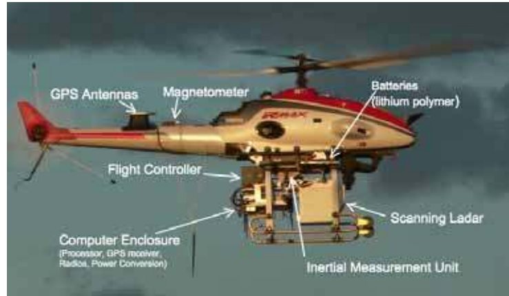
Figure 17: The helicopter testbed, a Yamaha RMax, used for our experiments has a payload of 29kg + fuel.
