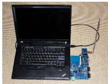
Figure 3: Data collection setup based on the SI-4735 FM radio receiver from Silicon Labs and the Intel WiFi Link 5300 wireless card connected to a Lenovo T61p laptop.
