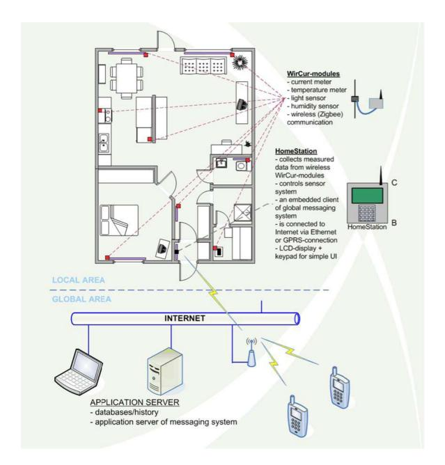
Different terminals or equipment are same level peers of the system as the data storing terminal, also one or more software agents for autonomic computing and data saving to database are same level peers of the system. WWW (World Wide Web) command and control UI (user interface) is provided using software agent as a gateway. Communication between peers is routed confidentially and securely. Dynamical WWW pages offer different
