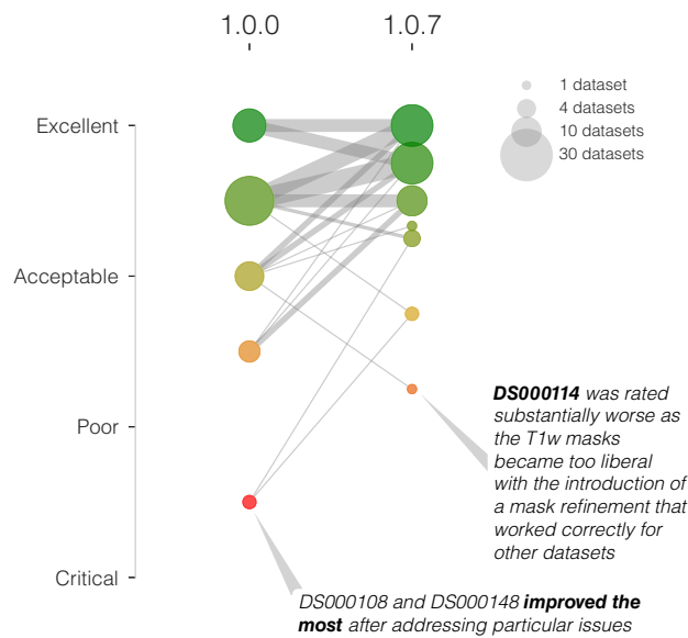
Figure 4. Integrating visual assessment into the software testing framework effectively increases the quality of results. In an early assessment of quality using fMRIPrep version 1.0.0, the overall rating of two datasets was below the “poor” category and four below the “acceptable” level (left column of colored circles). After addressing some outstanding issues detected by the early assessment, the overall quality of processing is substantially improved (right column of circles), and no datasets are below the “poor” quality level. Only two datasets are rated below the “acceptable” level in the second assessment (using fMRIPrep version 1.0.7).
