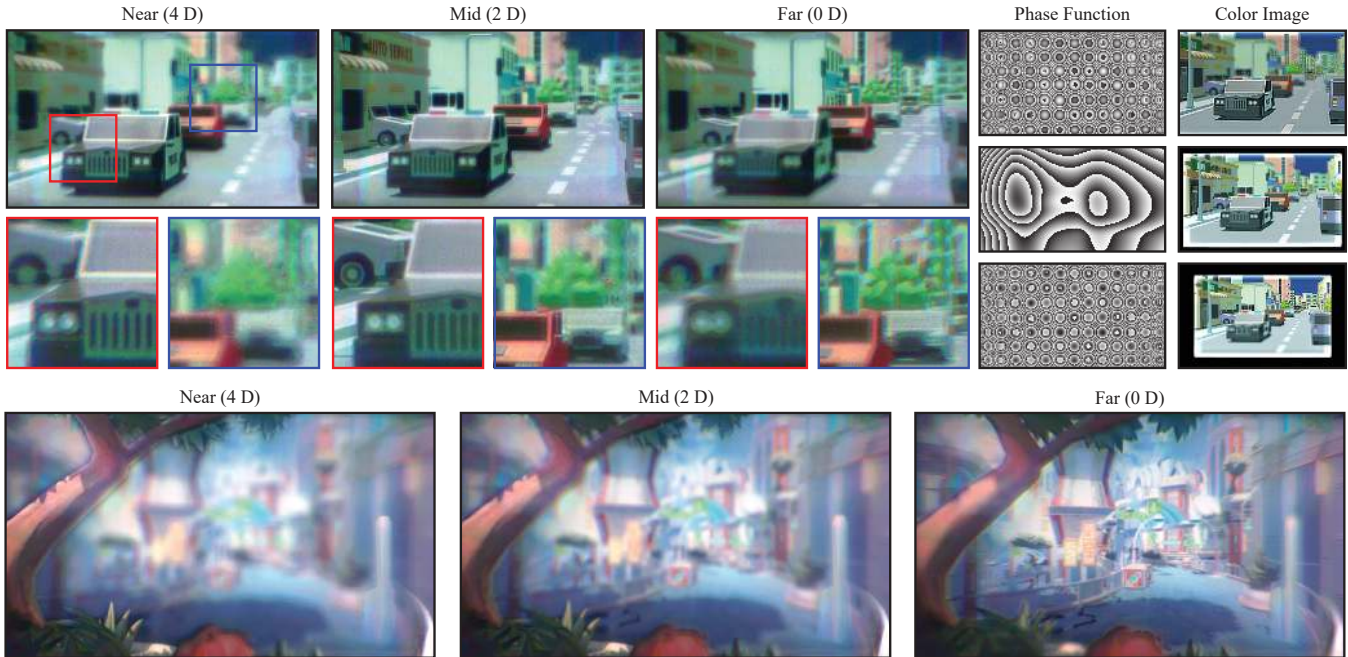
Fig. 11. Our prototype focal surface display achieves high resolution with near-correct retinal blur. Photographs of the prototype are shown in the first three columns, as taken by focusing the camera at the indicated distances. The last two columns depict the corresponding optimization outputs, including the phase functions and the color images. Note that optimized blending is applied with three time-multiplexed focal surfaces. The phase functions are wrapped assuming a wavelength of 532 nm. Note that the results for the lower scene employ linear blending, following Akeley et al. [2004]. See the supplementary video for the full focal stack results. (Source imagery courtesy Unity Asset Store publisher “VenCreations” and Thomas Guillon.)
