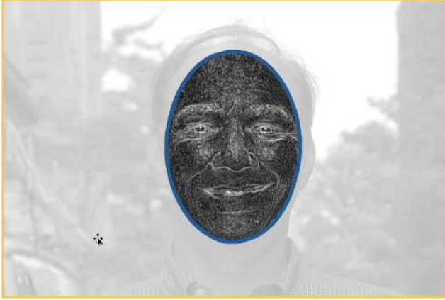
Figure 3. Face Region In Focus Measure (FRIFM) values are computed by summing edge density within an oval face mask.
