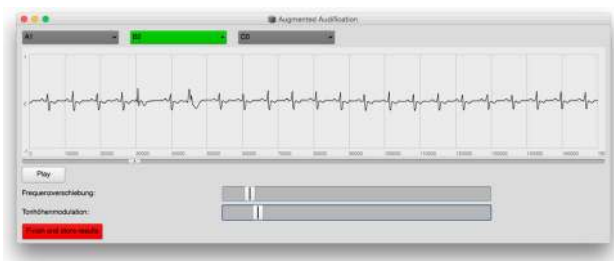
Fig. 5 Graphical user interface used in the pilot test. Subjects could choose out of nine sound files sorted in three groups (anonymously labeled A0–C3). The waveform was shown with a reference of the position of the data readout. (The graphics show aliasing which is usual for cardiologists and was therefore not adjusted. We indicated this fact to the subjects.) Two sliders without numerical reference and with simple labeling (“Frequency shift” and “Pitch modulation”) could be adjusted freely
