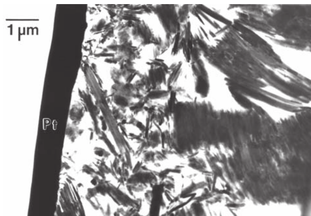
FIGURE 6. A bright-field TEM image of a FIB-milled kaolinite section with Pt strap.
