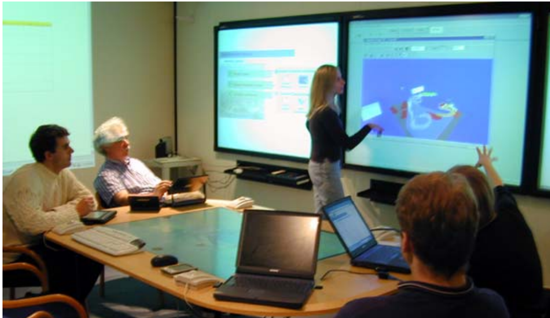
FIG. 5: Interactive Workspace consisting of several interactive touchscreens, a table display, and other information devices such as laptops, PDAs, cameras, scanners, etc. Specialized input and output devices such as LCD-tablets, laser pointer trackers, microphone arrays and pan-and-tilt cameras are also present in the
