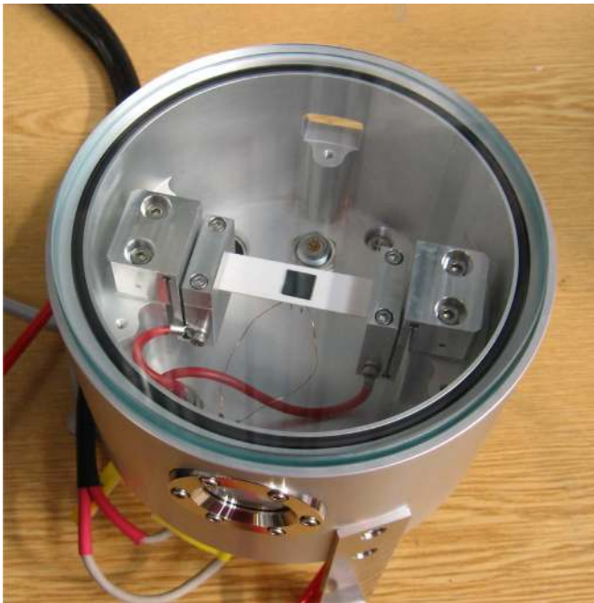
Fig. 9. Furnace for in-situ/in-operando annealing. The beam enters and leaves the recipient through sapphire windows. The 1\text{ cm}^2 sample is visible as a dark square on the white resistive heater bar.
