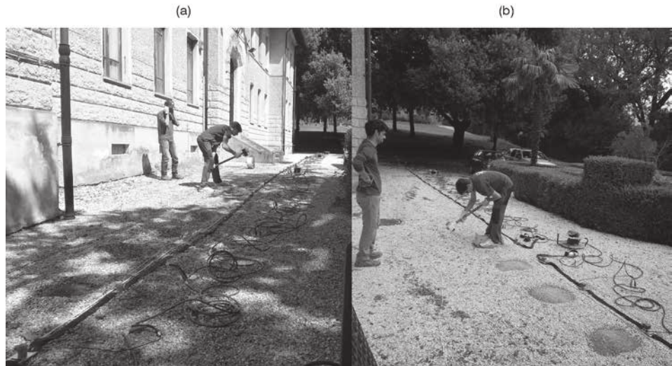
Figure 4 (a) P-wave and (b) SH-wave acquisition on the L1 line.
