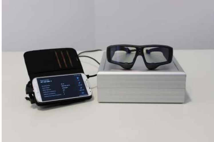
Fig. 1 Mobile eye-tracker glasses (SMI ETG, SensoMotoric Instruments GmbH (SMI), Germany) used for recording
