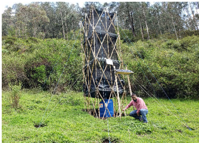
Fig. 13. Fog collector sistema in operation
