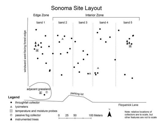
Figure 1. Sampling locations of instrumented trees (tree symbol ♠), throughfall collectors (●), soil moisture and temperature probes (squares ■), zero-tension and tension lysimeters (triangles ▲), and fog collector (F), redwood forest in Sonoma County, CA. round. Fog water was collected outside the forest using a passive fog collector with a plastic mesh collection surface (after Azevedo and Morgan 1974).
