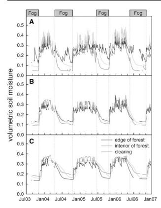
**Figure 3.** Volumetric soil moisture (as measured by TDR probes) by location within a redwood forest stand in Sonoma County, CA (open, edge zone, interior zone, see Figure 1) and soil depth (**A**) 0–10 cm, (**B**) 35 cm, (**C**) 70 cm from August 2003 to December, 2006.
