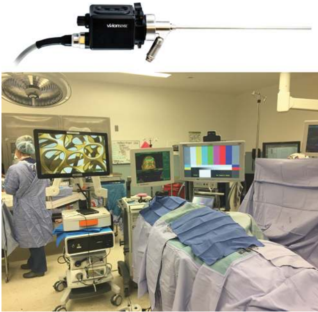
FIG. 1. Visionsense equipment setup for NIR imaging. Upper: The excitation laser for NIR imaging is attached to a 4-mm endoscope. Copyright Visionsense. Published with permission. Lower: Images are displayed on the leftmost screen. Figure is available in color online only.
