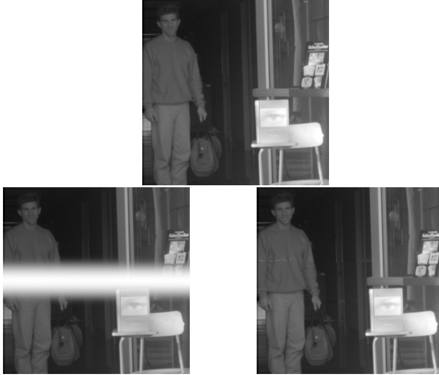
Figure 6. Top: Image of HDR scene. Bottom left: Simulated image with moving laser. Bottom right: Simulated image using FMC with disturbance tolerance.
