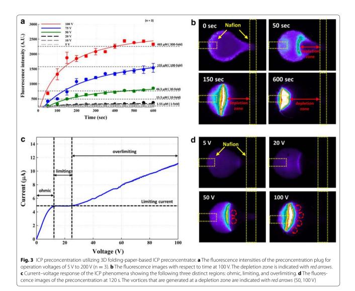
We observed 100 V, the optimal electric potential that we operated for ICP, are in the overlimiting region that generates vortices of electroconvection.
