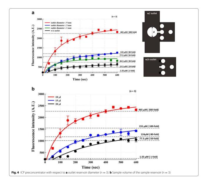
volumes of 10  $\mu$ L (red line), 15  $\mu$ L (blue line), and 20  $\mu$ L (black line), respectively. In general, the preconcentrating volume and factor have been considered as a trade-off. If the preconcentrating volume is increased, the preconcentrating factor generally decreases. In Fig. 4b, a higher preconcentrating factor is observed for a total preconcentration volume of 10  $\mu$ L.
