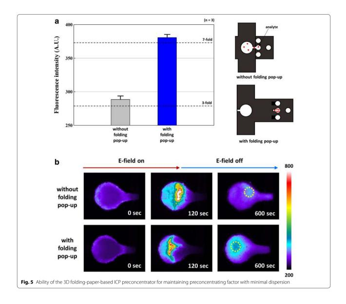
small dispersion, as the capillary forces were eliminated by disconnecting the fluidic channel.
