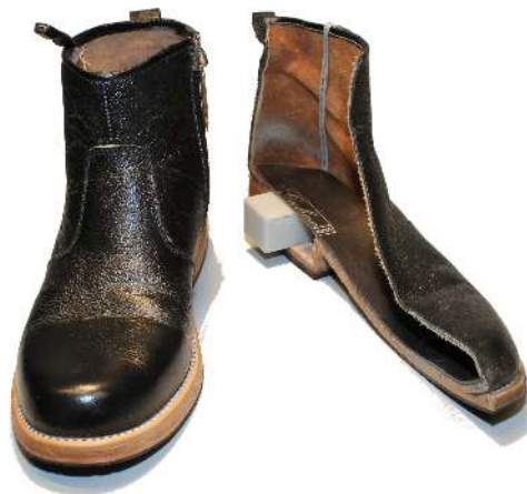
Fig. 1: Shoes with units of the presented foot-mounted INS implementation integrated in the heels and cabling with USB connectors at the shoe shafts. The cabling inside the shoes is normally protected by a leather patch but is here displayed for clarity.
