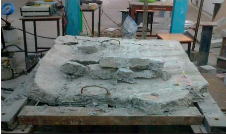
FIGURE 13: Final brittle collapse of glass fiber reinforced paper mass slab.
