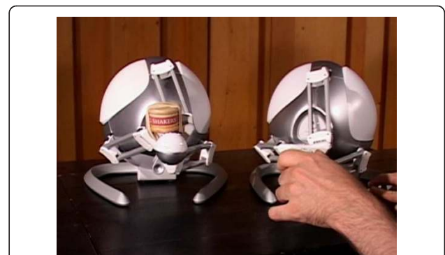
Figure 10 Force-feedback device plays a musical shaker on the left as directed by a human conductor via the force-feedback device on the right.
