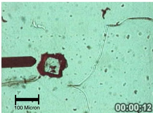
Fig. 6 Microscopic view of the pusher and the micro-object
