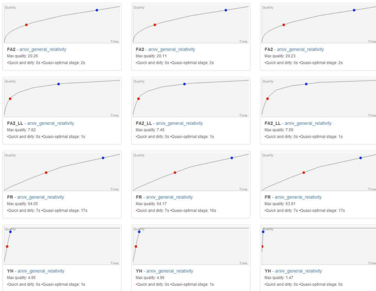
Figure 10. Records for a single network. Evolution of the layout quality for a single network over 2048 steps. Rows are the 4 different layouts and columns the 3 different randomizations. The red dot is the “Quick and dirty point” where 50% of the maximum quality is reached, and the blue dot is the “Quasi-optimal point” where 90% of the maximum quality is reached. The full visualization is available at this URL: https://github.com/medialab/benchmarkForceAtlas2/tree/master/benchmarkResults . doi:10.1371/journal.pone.0098679.g010
