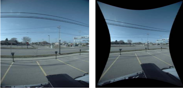
Fig. 6. The left panel shows a spherically distorted image obtained from the Ladybug3 camera. The right panel shows the corresponding undistorted image obtained after applying the transformation provided by the manufacturer.
