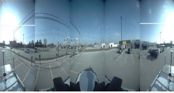
Fig. 5. The distorted images, from the five horizontal sensors of the omnidirectional camera, stacked together.
