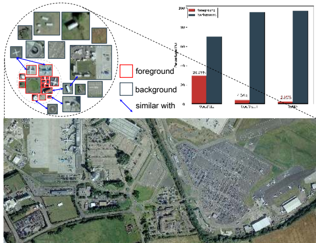
Figure 1. The main challenges of object segmentation in the HSR remote sensing imagery. (1) larger-scale variation. (2) foreground-background imbalance. (3) intra-class variance of background.
