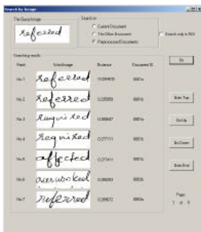
Fig 3. Cropped Word image as query to the digital library; all the similar word images are returned as a ranked list.
