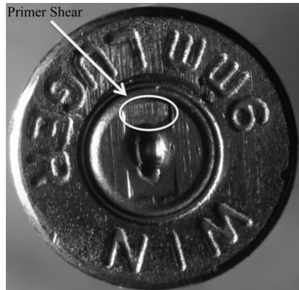
Fig 1. Primer shear. Striation pattern produced by shearing action of breech face of Glock 19 against the cartridge case primer.
