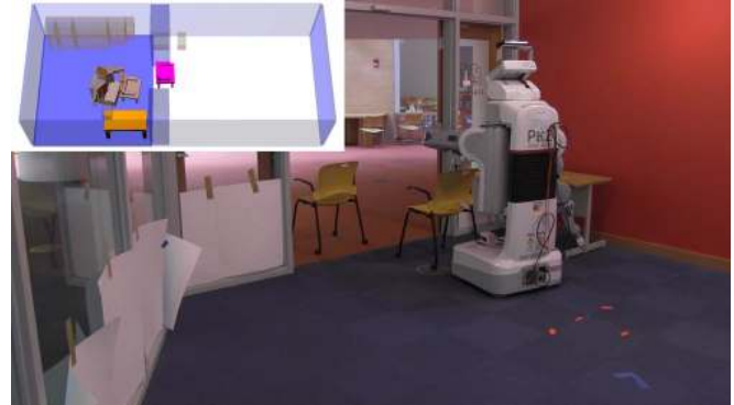
Fig. 1. Solving a NAMO problem with a PR2. The robot discovers two unknown obstacles (chairs) and moves them out of the doorway in order to get through.
