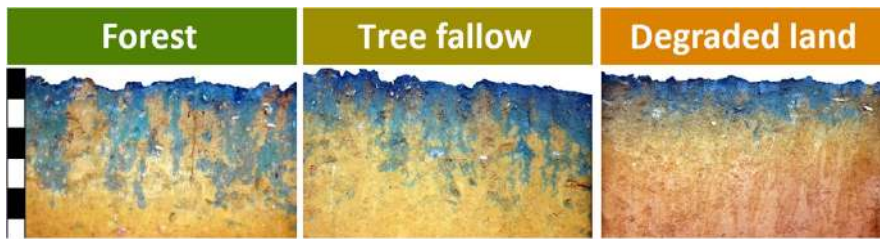
FIGURE 4 Example pictures of the blue dye profiles showing preferential flow for three nearby sites in the western study area. Each block on the black and white scale bar represents 10 cm
