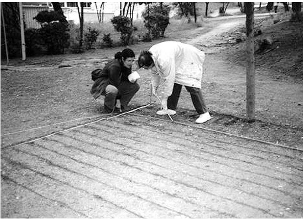
Figure 7. Preparation of the grid of profiles near an isolated tree.
