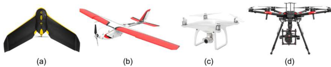
Figure 4. Some of the most used unmanned vehicle types: (a) fixed-wing, SenseFly eBee; (b) PrecisionHawk Lancaster; (c) rotary-wing, DJI Phantom 4 and (d) DJI Matrice 600 Pro.
