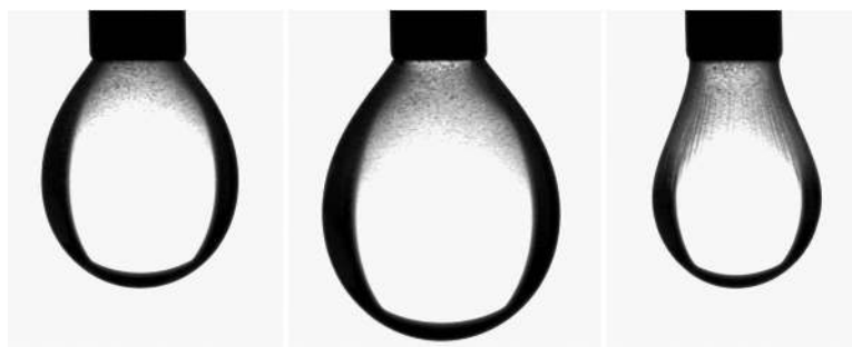
Figure 3. Images of crosslinked G92 copolymer membrane (20 minute incubation) during the 1st expansion/compression/expansion cycle. The left image corresponds to A/A_0=1 , where A_0 is the drop surface area at the beginning of the cycle. The center image corresponds to A/A_0=1.39 (maximum surface area during cycle). The right image corresponds to a deep compressed state ( A/A_0=0.81 ) where wrinkling can be observed in the upper portion of drop interface.
