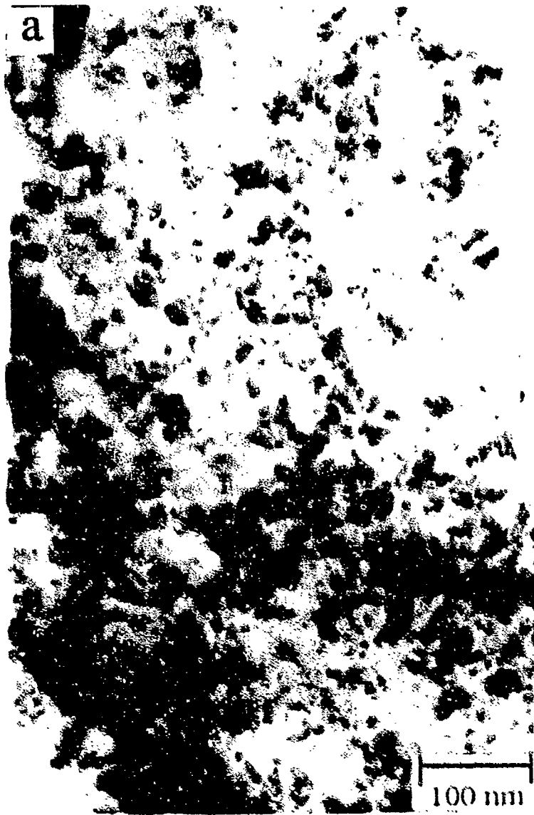
Figure 9a. TEM bright field micrograph of shear band material in the N-925 microstructure.
